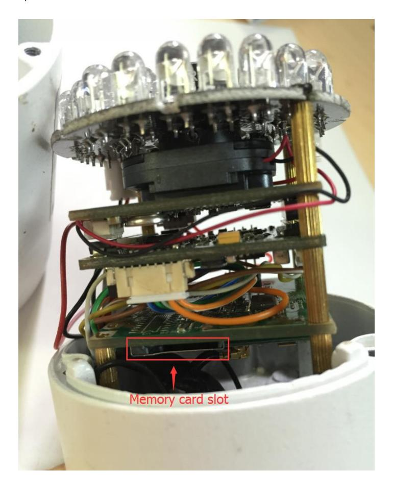
3, Insert SD card, assemble camera housing.
